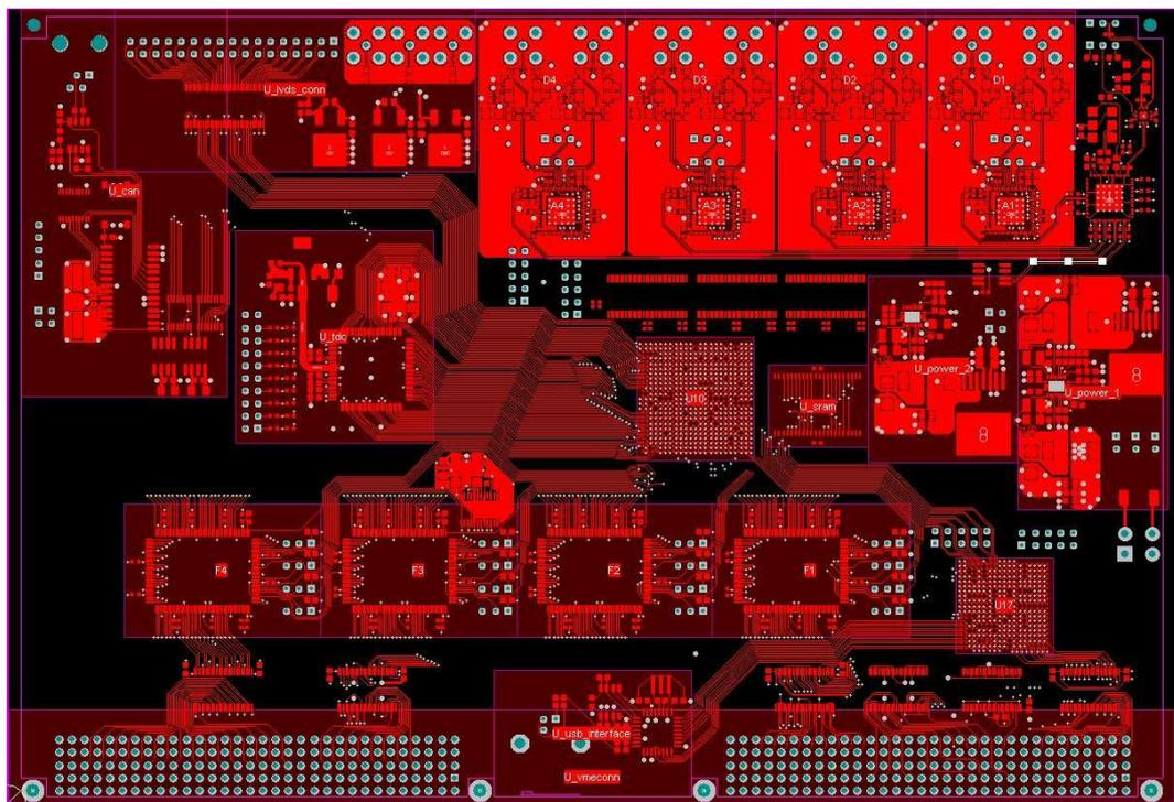
Figure 8: Top layer of the Neutrino DAQ printed circuit board.
