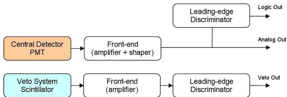
Figure 1: The signal path from the detectors to the Data acquisition System.
