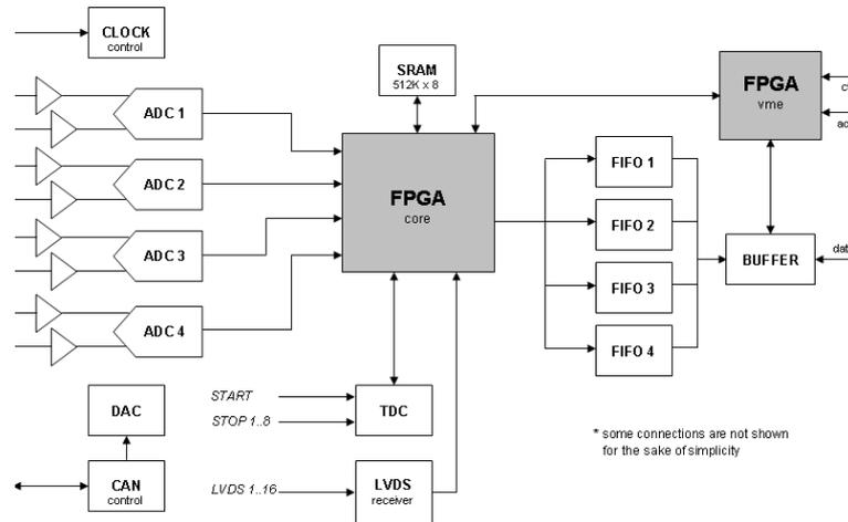
Figure 5: Neutrino DAQ module diagram
