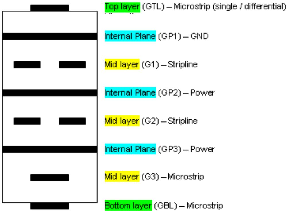
Figure 7: Layer stack of the NDAQ module.
