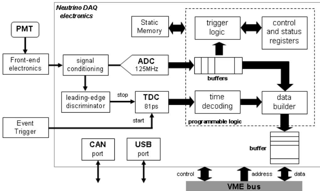
Figure 4: Basic processing blocks of the Neutrino-DAQ (one channel).
