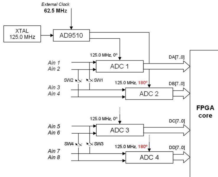
Figure 6: Analog-to-Digital Conversion scheme for 250 MHz sampling.
