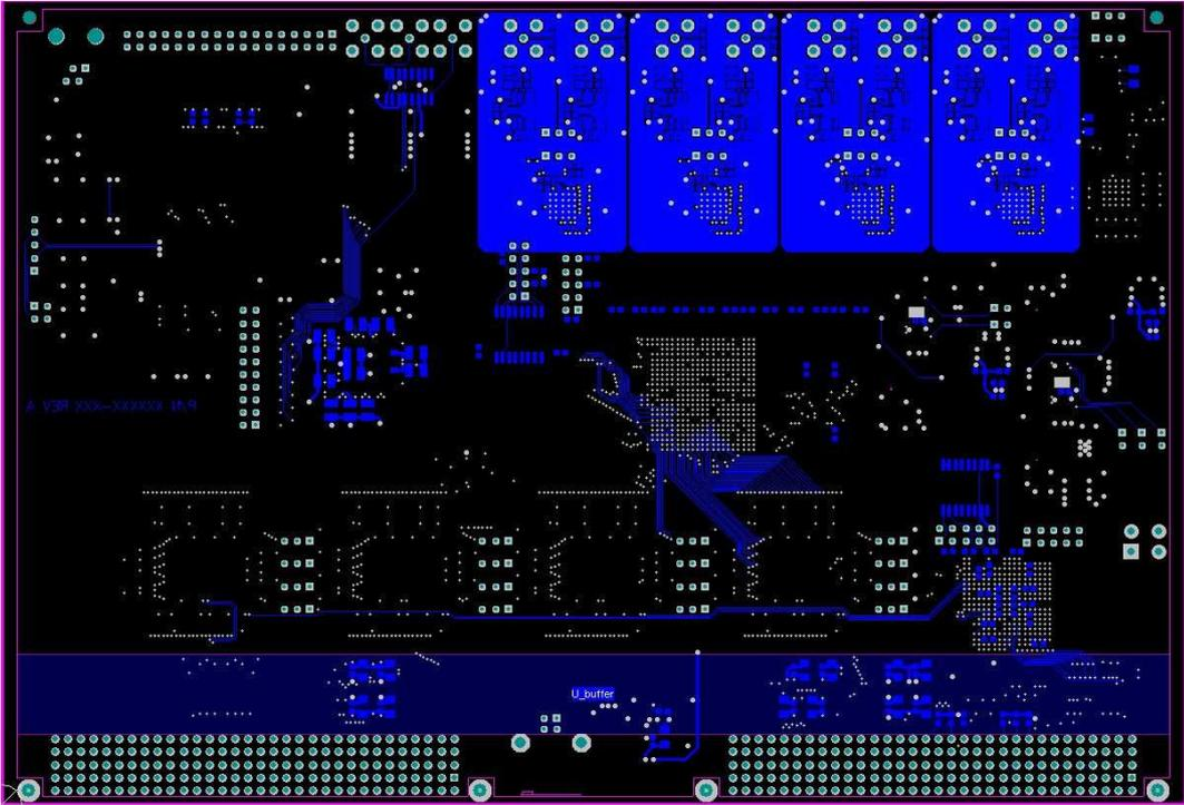
Figure 9: Figure 9: Bottom layer of the Neutrino DAQ printed circuit board.
