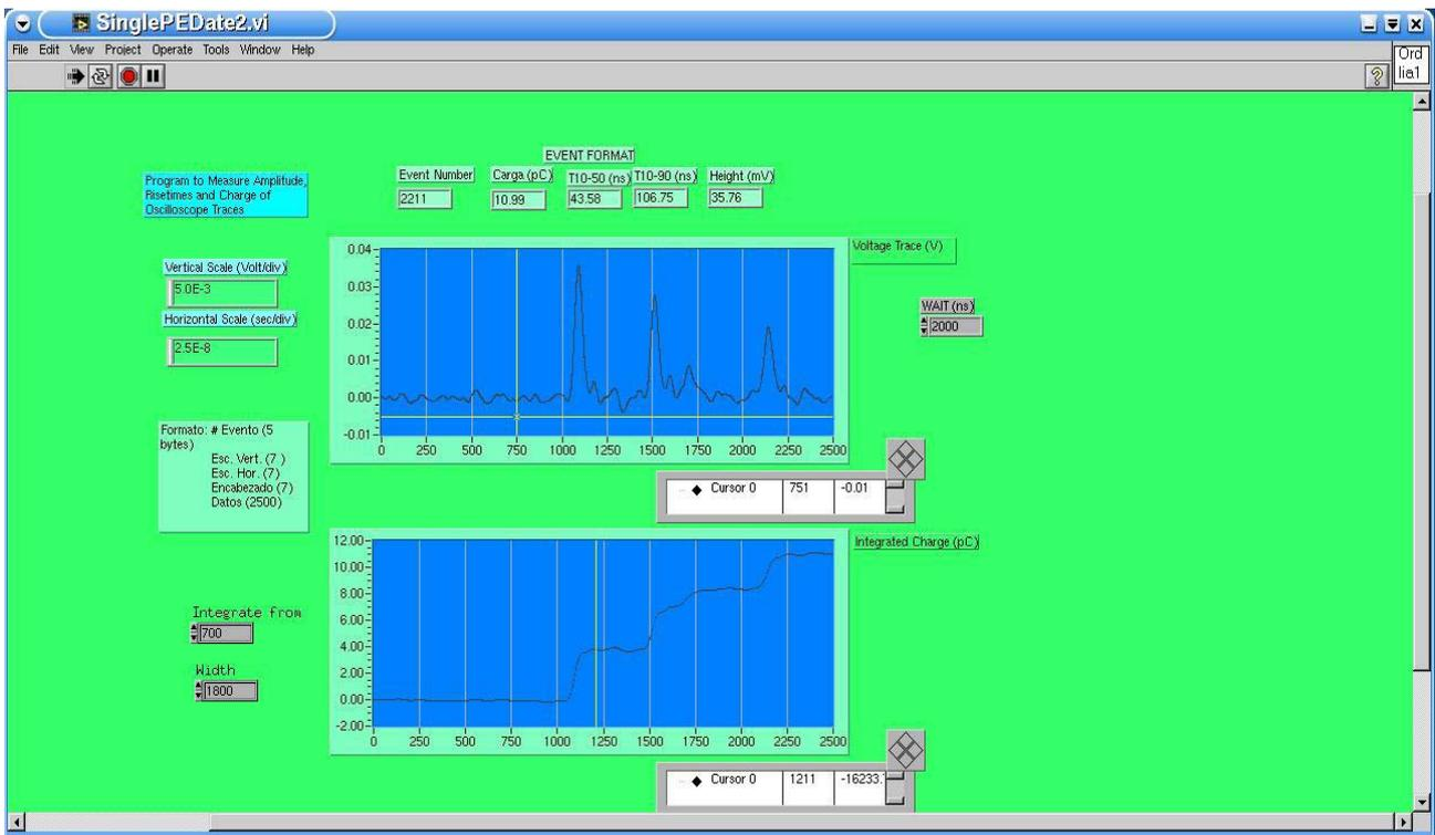
Figure 8: Event with three isolated PMT pulses. The upper curve is the PMT trace in V and the lower one the charge in pC. The horizontal scale is 25 ns/div.
