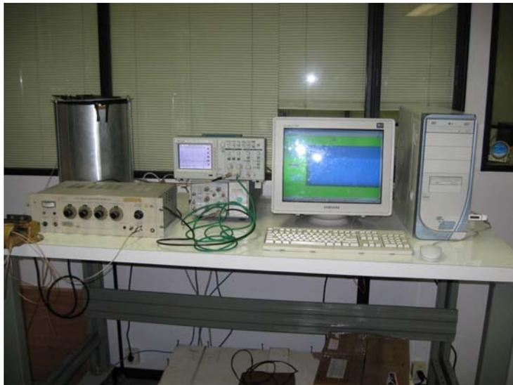
Figure 2: Experimental setup photograph, from left to right: dark chamber with the PMT and LED inside; HV power supply Keithley 246; pulse generator Tektronix PG508; digital oscilloscope Tektronix TDS 1012B; IBM personal computer, with Microsoft Windows XP.
