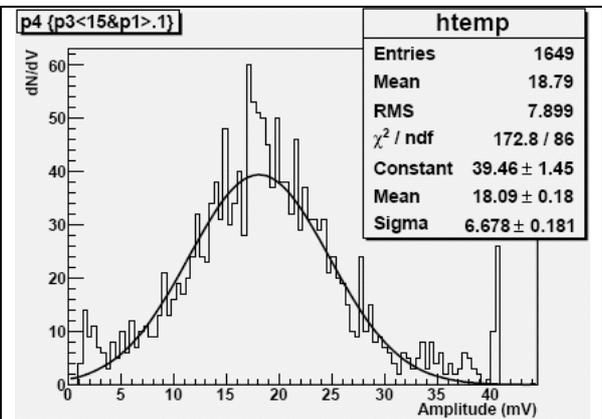
Figure 13: Pulse amplitude for events with  $Q > .1$  pC and  $risetime > 15$  ns.
