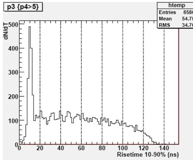
Figure 11: Risetime for events with  $V > 5$  mV. The single peak between 0 and 15 ns corresponds to single photoelectron pulses, the flat distribution above 15 ns is due to our using a slow LED.
