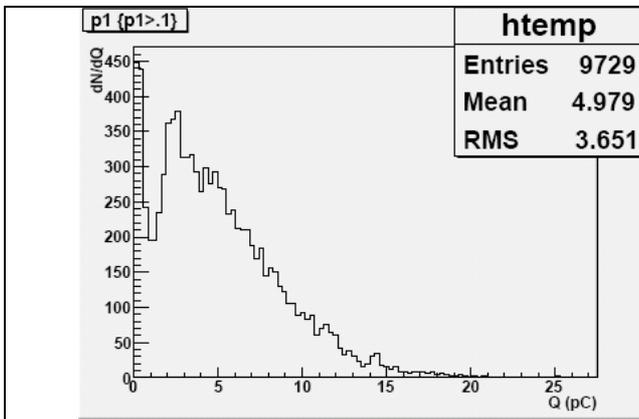
Figure 12: Pulse amplitude for events with  $Q > .1$  pC and  $risetime > 15$  ns.
