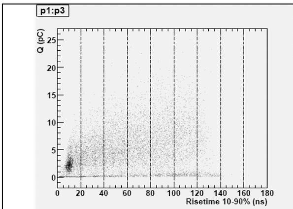
Figure 9: Charge vs risetime from 10 to 90% for a set of events taken on August 31th., 2007.
