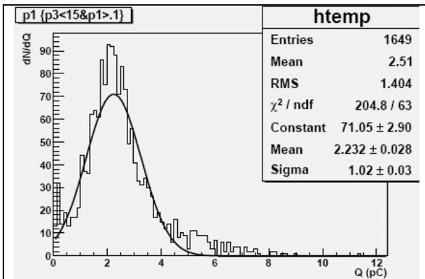
Figure 14: PMT charge for events with  $Q > .1$  pC and  $risetime < 15$  ns.
