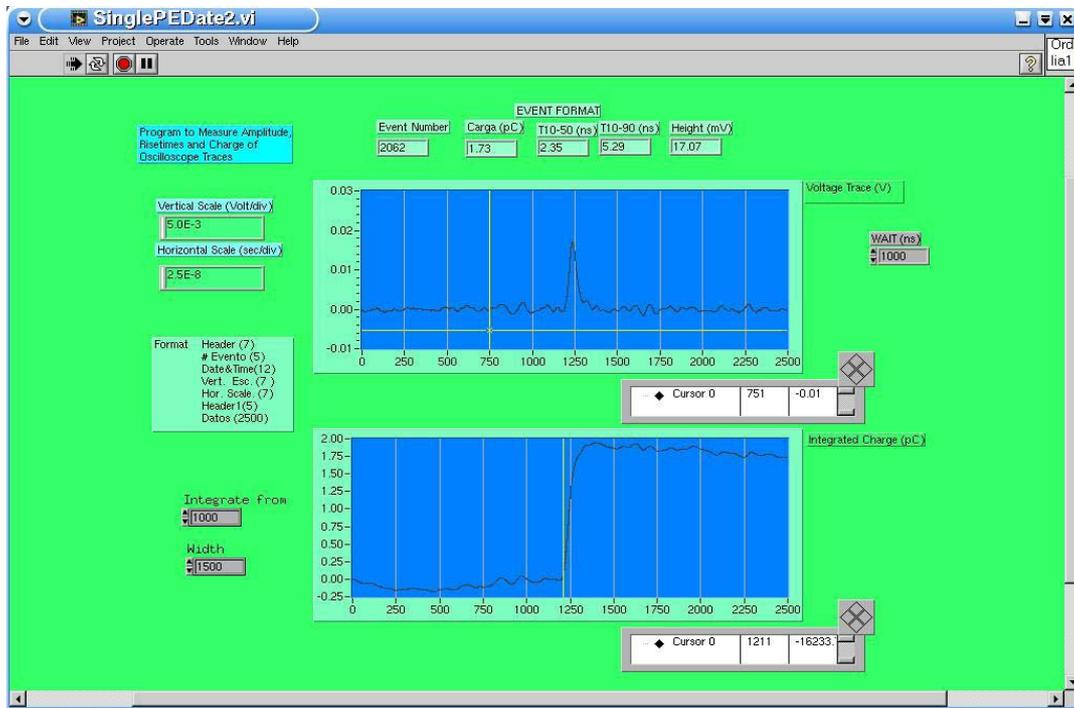
Figure 6: Event with a single isolated PMT pulse. The upper curve is the PMT trace in V and the lower one the PMT output charge in pC. The horizontal scale is 25 ns/div.
