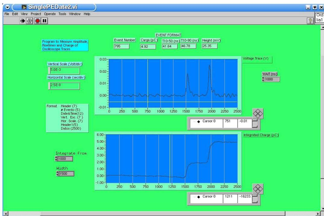
Figure 7: Event with two isolated PMT pulses. The upper curve is the PMT trace in V and the lower one the charge in pC. The horizontal scale is 25 ns/div. are measured. Therefore, the technique illustrated in this note can be applied to PMTs with gains well below 107, where it would be impossible to measure gains with a commercial ADC because the typical 0.25 pC resolution is inadequately coarse.
