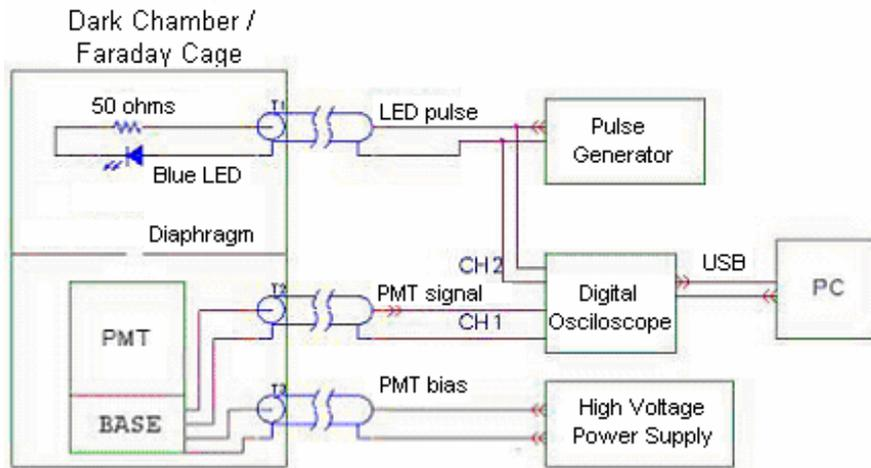
Figure 1 – Setup schematic diagram
