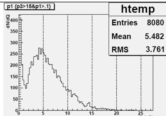
Figure 15: PMT charge for events with  $Q > .1$  pC and  $risetime > 15$  ns. The most probable value is twice that of a single PE.
