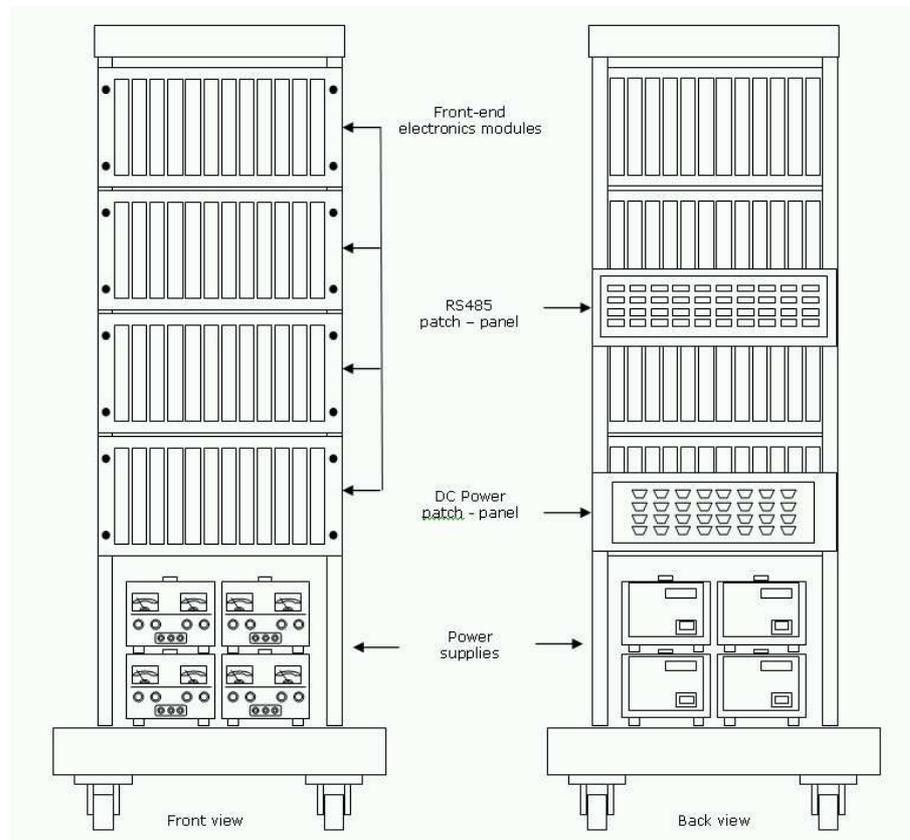
**Figure 3:** Sketch of the setup of racks with front-end modules, power supplies, and patch panels for DC power output and RS485 connections.
