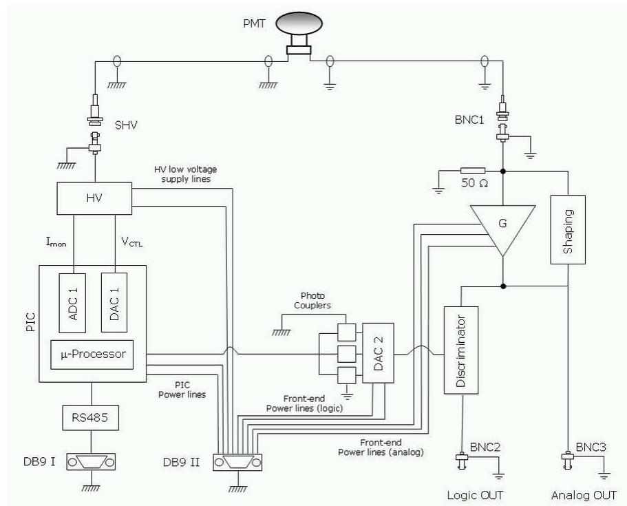
Figure 2: General view of the circuit blocks composing the front-end electronics system.
