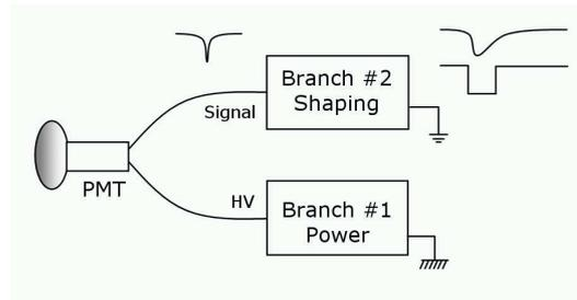
Figure 1: The two electronics branches assigned to each PMT.
